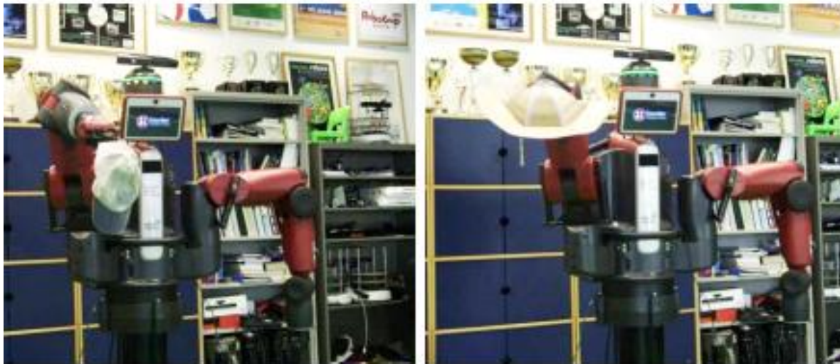
Fig. 1: Baxter manipulator ready to help dress a user with two different hats
