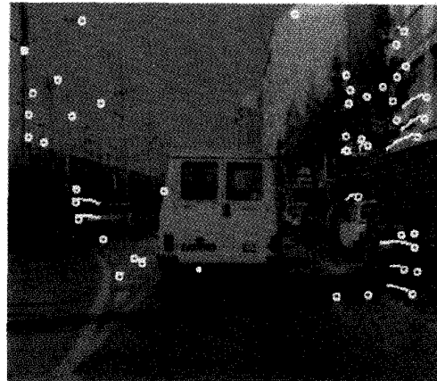
Fig. 15. Corner trajectories with 4 or less actual measurements tracked through the "J7" sequence up to Frame 55 with N -scan lookahead set to zero.
