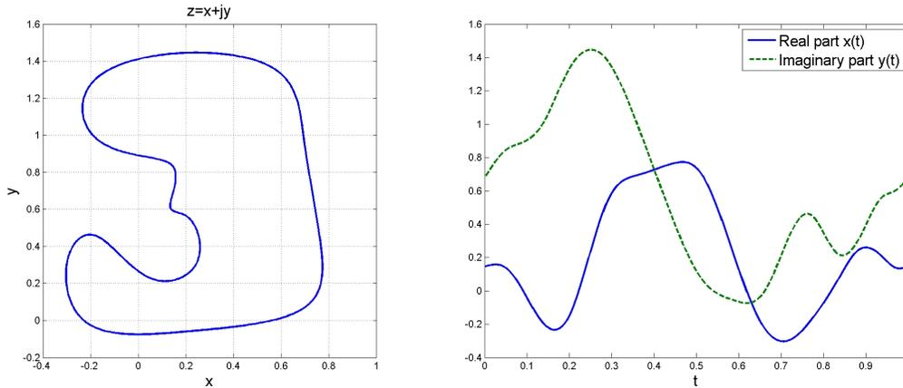
Figure 13: A contour as a periodic signal in the complex plane.
