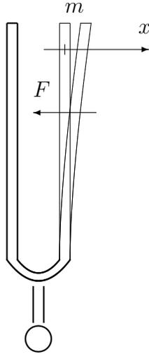
Figure 4: Vibrating tuning fork model.
