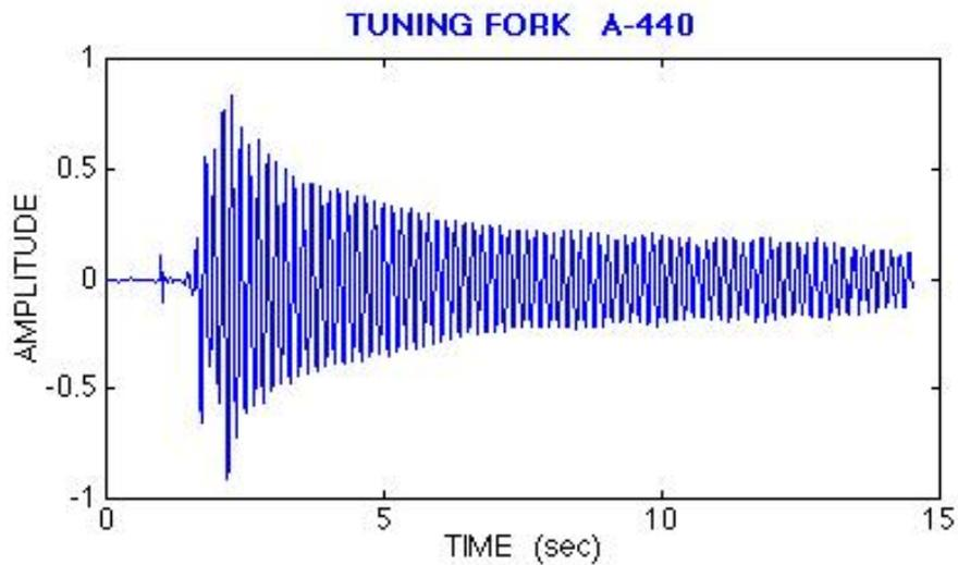
Figure 2: Acoustic signal produced by a tuning fork. (From [1].)
