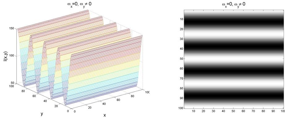
Figure 9: Sinusoidal image. Left: image intensity as a function of  $x$  and  $y$ . Right: corresponding gray level image.
