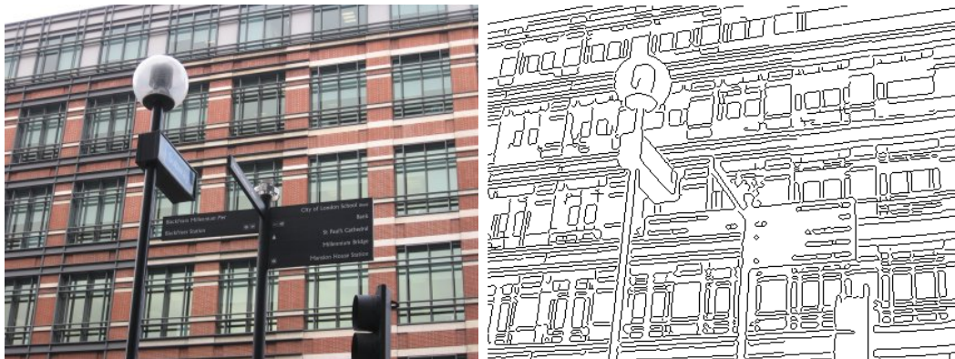
Figure 1.2: Complex image with dense clutter and the poor response of the Canny edge detector. Left: image; right: the detected edges (note the many missing edges)
