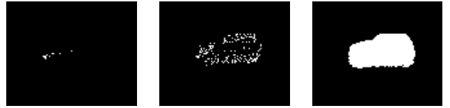
Fig. 4. Three stages of the relaxation process for the video sequence illustrated in Fig. 3. The final estimate of the moving object template is on the rightmost image.
