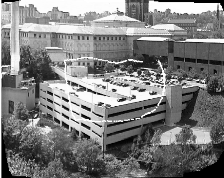
Figure 2.10 The background mosaic for the “Oakland” sequence. It also shows the trajectory of the camera center as it moves to capture the 300 frames. (Source: From R.S. Jasinski, J.M.F. Moura, J.C. Cheng, and A. Asif, Proceedings of IEEE ICASSP, 1995.)
