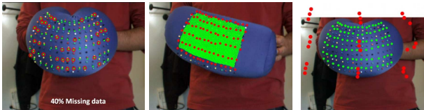
Figure 1. Cushion sequence results. Starting from the left image we have the 2D original image tracks with missing data, the reprojected dense mesh in green and the control points location in red.
