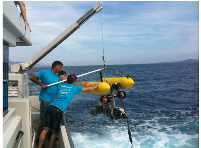
Fig. 4. The lightweight AUV GIRONA500 being deployed from the 24m R/V *Bon Pigall* above the *La Lune* shipwreck.
