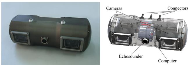
Fig. 3. High resolution stereo imaging system.
