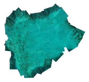
Fig. 3. Final mosaic for the first image sequence. It was created using 129 images selected from the original set of 1000 and rendered with the *closest* operator. The seafloor area covered is approximately  $42 m^2$ .
