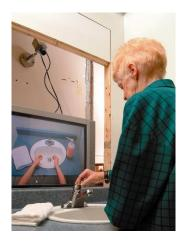
An intelligent cognitive device that tracks a user through handwashing, providing cues when necessary.
