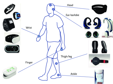
Figure 7 - Location on the body of several commercially available wearable devices. (Image source [11])
