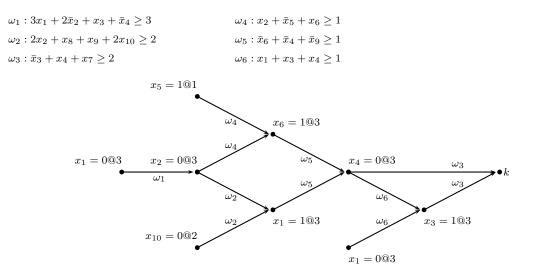
Figure 3.2: Example of a PB formula, a partial assignment, a decision assignment and the corresponding implication graph
