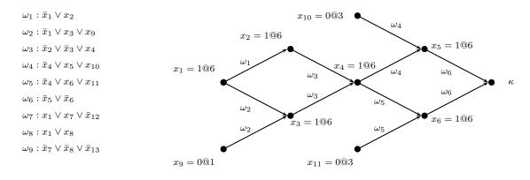
Figure 2.2: Example of a formula, an assignment and the corresponding implication graph
