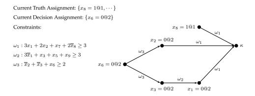
Figure 3.4: A PB formula, a PB partial assignment and the corresponding implication graph
