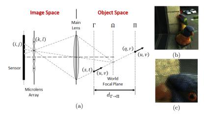
Fig. 2. Geometry of a SPC whose main lens focal plane corresponds to plane  $\Omega$  (a). The LF in the image space is parameterized using pixels (i, j) and microlenses (k, l) indices while the LF in the object space is parameterized using a point (s, t) and a direction (u, v) defined on the parameterization plane  $\Gamma$ . (b) shows a raw image acquired with a SPC with the mains lens world focal plane placed near the wall and (c) exhibits the details of the microlenses in red box A.
