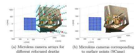
Fig. 3. Microlens camera arrays obtained considering shearing for refocusing at different depths for the synthetic Table dataset [9]. Shearing allows to obtain microlens cameras with projection centers at different depths (a). These cameras obtain relevant information for depth estimation [5] when the projection center corresponds to a surface point, *i.e.* a SCam is defined (b). The viewpoint camera array is represented in blue with the spacing among projection centers scaled by 4 times.
