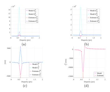
Fig. 5. Variation of microlens camera intrinsic matrix and projection center with disparity  $\beta$  for shearing. These entries are estimated considering that  $\Delta k = \Delta l = 1$ . The scale factors of the intrinsic matrix  $k_{11}^{kl}$  and  $k_{22}^{kl}$  are represented in (a). The principal point  $\left[k_{13}^{kl}, k_{23}^{kl}\right]^T$  is depicted in (b). The *x*- and *y*- components of the projection are presented in (c) while the *z*-component is presented in (d).
