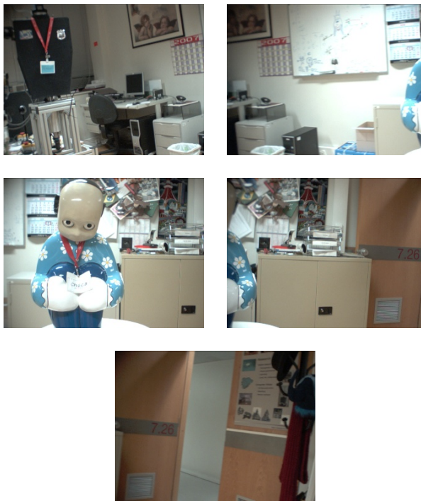
Figure 2. Exploring an empty laboratory with threshold = 0.7 resulted in 5 image clusters being saved before stabilizing the system. Such a low number of classes was expected, given the rather uniform colours in the environment.
