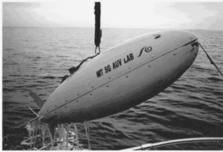
Fig. 1. An Odyssey IIB AUV being recovered after operations.
