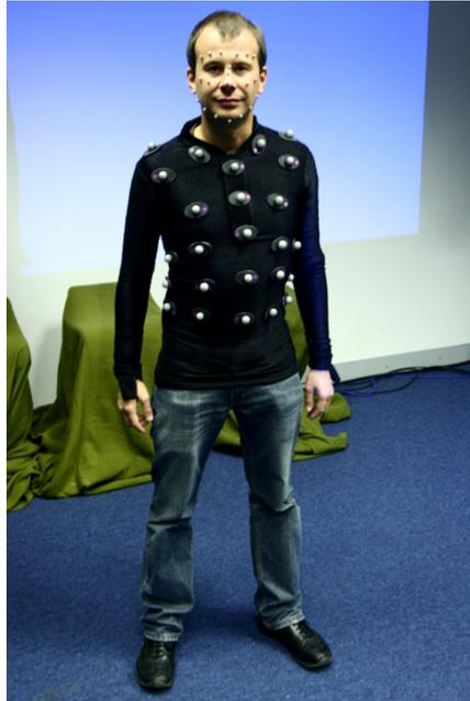
Figure 1.1: Example of a marker setup for a MOCAP analysis.
